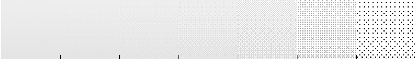
Figure 4: The same gray quantized and dithered from 7 bpc (left) to 1 bpc (right). At lower bit depths, a perceptual lightness shift emerges, appearing progressively “whiter”. This effect is primarily caused by the sparse palette from quantization.
