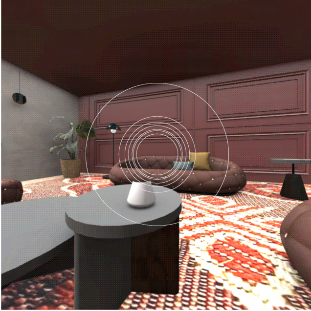
Figure 9: Foveated mask with mean thresholds from the study. Settings match the bottom line in Figure 8.
